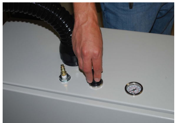
Air Regulator to set Gripper Wheel Pressure
